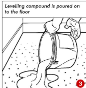
Holes or uneven patches can be filled with a self-levelling compound which is poured on the floor and spread out with
