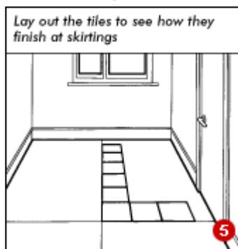
For the best appearance, establish how the tiles are to be set out beforehand. Avoid leaving narrow strips along skirtings and especially at a doorway (5).
